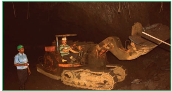
Side Discharge Loader installed at mine
