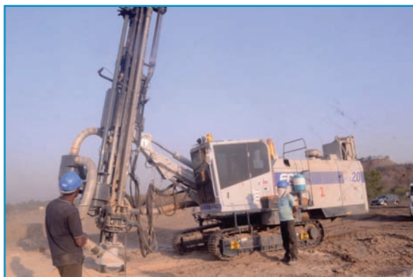
Furukawa make heavy duty wagon drill machine
