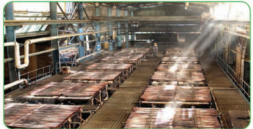
MOIL'S ELECTROLYTIC MANGANESE DIOXIDE (EMD) PLANT OF 1000 TPA CAPACITY AT DONGRI BUZURG MINE
